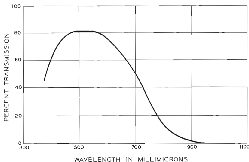
FIG. 6. Transmission characteristics of infrared filter combination.
