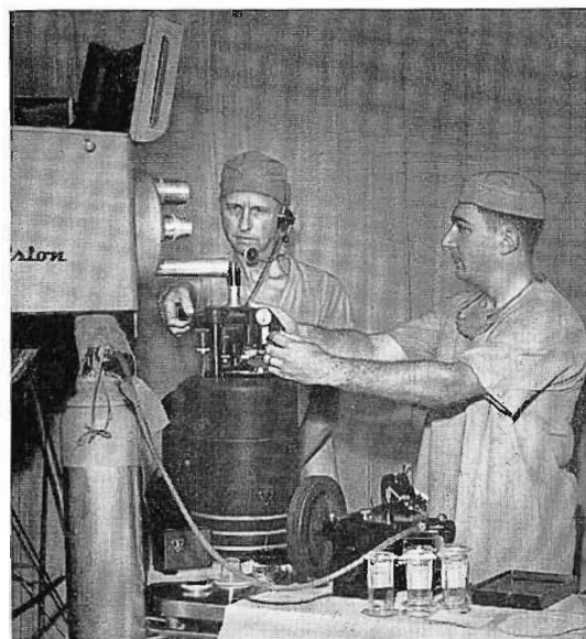
BIOPSY. Slide of prepared and tested specimen is placed in microprojector and viewed by TK-41 Camera.
