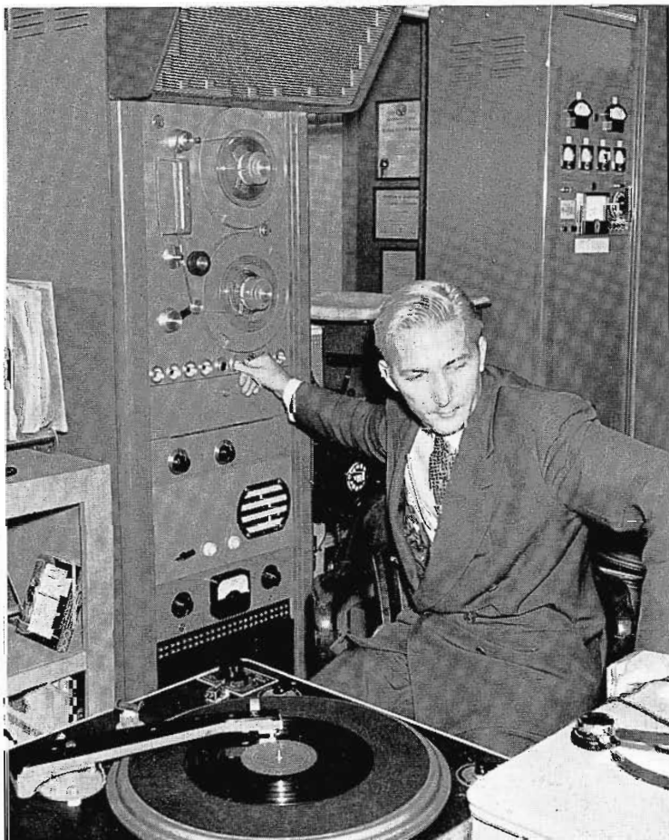
John F. Moore, Station Manager, demonstrates operation of RCA RT-11B tape programming equipment.
